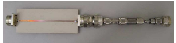
Fig. 12. Network used to verify the technique of predicting the IM distortion product of a system due to coaxial connectors.
